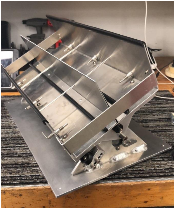
This is a Fly Sleep Deprivation device (researchers put fruit flies into a fixture with some tubes and this machine keeps them awake). The In-House Fabrication Team completed this project in support of researchers at the University of Missouri – Kansas City.
